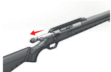
Picture 18: By pulling the bolt rearward and forward again, a cartridge placed into chamber. Pull the bolt down clockwise to lock.
