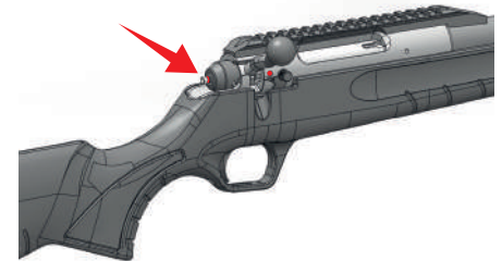
Picture 4: Cocking the firing pin.
