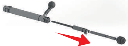
Picture 8: Spring in the firing pin assembly will push the firing pin and follower outside of the bolt.
