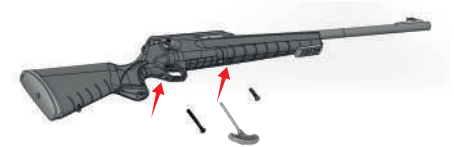
Picture 24: Two screws connecting receiver and stock should be removed.
