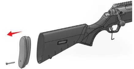
Picture 28: Butt plate is removed from the stock.
